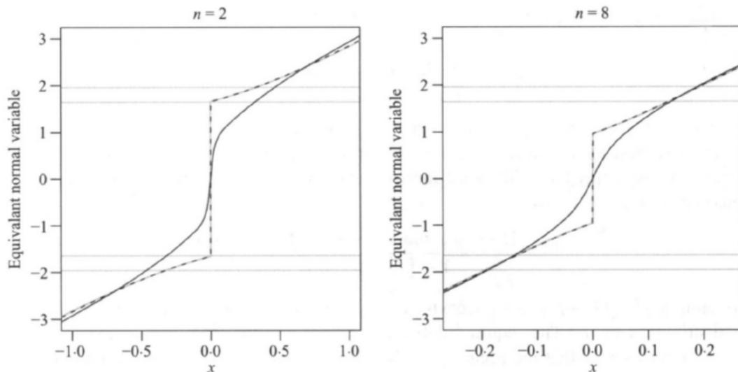
Fig. 1. Comparison of saddlepoint approximations  $\tilde{F}$  (solid) and  $\hat{F}$  (dashes) with exact distribution  $F$  (solid, grey), which is identical to  $\tilde{F}$ , for normal/point mass mixture, with  $p = 0.05$ ,  $\mu = 0$ ,  $\sigma = 1$  and  $n = 2, 8$ . For clarity, the vertical scale is the equivalent normal variable  $\Phi^{-1}\{F(x)\}$ . The horizontal lines correspond to probabilities 0.025, 0.05, 0.95 and 0.975.
